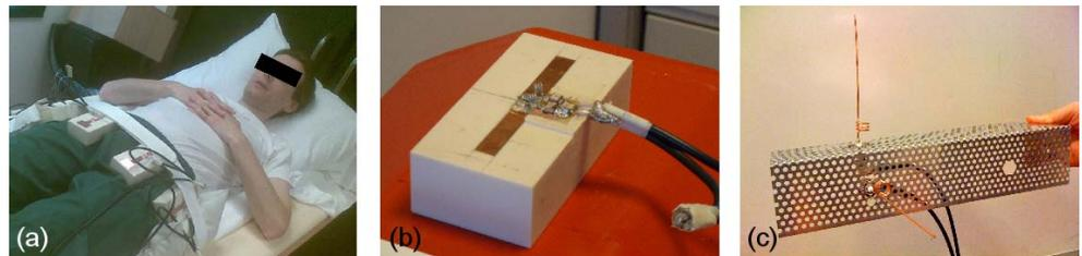
Figure 1: (a) Position of array elements on volunteer. (b) Single coil array element (c) SQL-antenna
