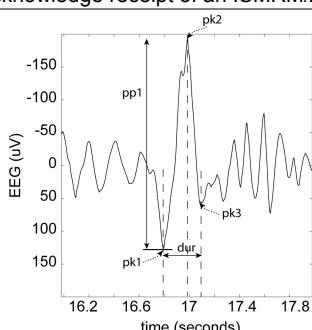
**Fig 1a.** Interictal EEG spike waveform. Timing-related and amplitude-related parameters are defined.
