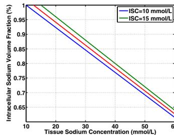
**Figure 1.** ISVF versus TSC plot. Imprecise knowledge of ISC causes small (less than 2%) error in ISVF measurement.
