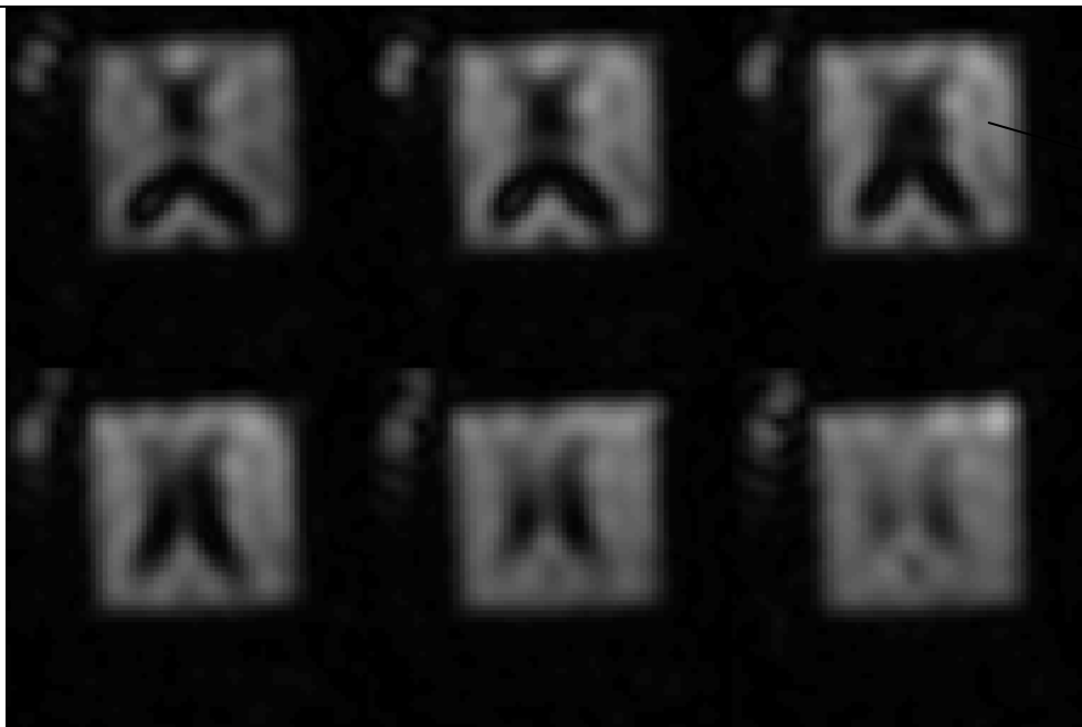
Fig 2: LASER-RSI Acquisition: NAA metabolite map (left) for a few slices. The effective in-plane resolution is 1cm x 1cm; both the x and y resolution were digitally enhanced (through zero-padding, before FT) by a factor of 4. The spectrum for a periventricular location (indicated by the arrow) is shown above.
