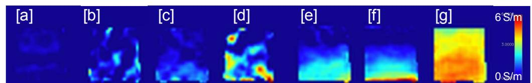
**Fig. 3** Series of SSFP real-time conductivity maps in tap water. [a] initial condition, [b, c, d] during addition of salt, [e, f] at three minutes intervals, [g] after stirring.
