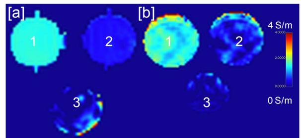
**Fig. 2** Color-coded coronal conductivity maps acquired with SE [a] and SSFP [b]. Three samples with phantom fluid (1, 2), and tap water (3) were used.
