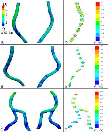
Figure 2. A-C) Time-averaged WSS distributions of Subjects 1-3, respectively (colorbar in A applies to A-C). D-F) Axial velocity contours in Subjects 1-3, respectively.
