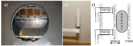
Fig. 1. Compression platform: a) coil carrying compression plates; b) syringe pistons; c) schematic
