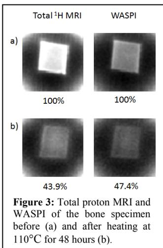
**Figure 3:** Total proton MRI and WASPI of the bone specimen before (a) and after heating at 110°C for 48 hours (b).
