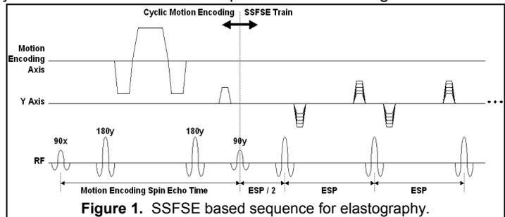
Figure 1. SSFSE based sequence for elastography.
