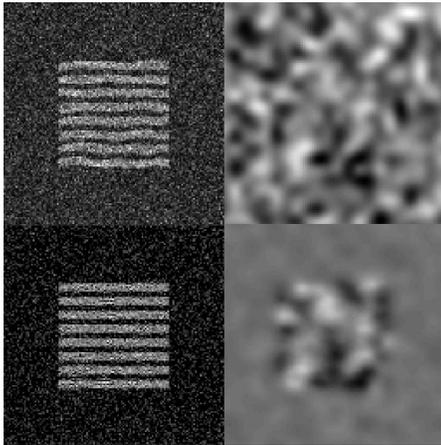
Fig 1: Top row: Distorted image and field used to distort it. Bottom row: Estimated undistorted image and field. Note how the noise floor has been reduced in the estimated image.
