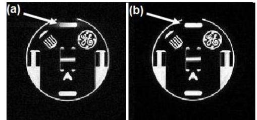
**Fig. 2.** Central slice of axial phantom dataset (SPGR) without off-resonance correction: (a) 3D stack-of-rings, (b) 3D concentric cylinders
