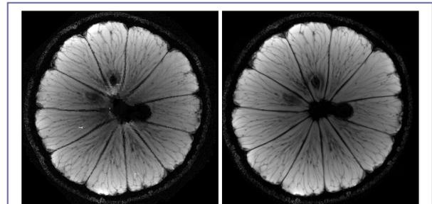
**Figure 2:** GRE images of a lemon using the new PatLoc gradient coil (left) and the linear gradient coil (right) for in-plane spatial encoding.
