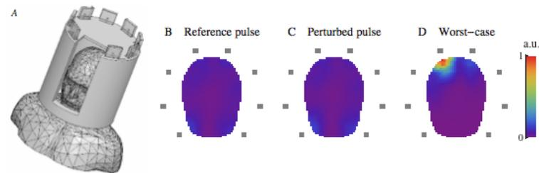
**Figure 1:** Simulation model, and axial slices containing the peak 10-gram SAR for a 3-spoke pulse. Coil positions are indicated with gray squares. A: Coil model as used in the simulations. B: SAR<sub>r</sub> distribution obtained using the reference pulse. C: the maximum SAR<sub>p</sub> found by introducing up to 20% amplitude perturbations and 20° in phase. D: the worst-case local SAR.
