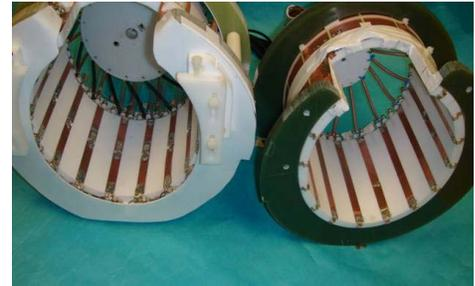
Fig.1 Photograph of the Z-shim array (left) and the 16 ch. array (right)
