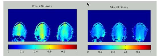
Fig. 4 RF Efficiency with the Z-shim array (left) and the 16 ch array (right) corresponding to the B<sub>1</sub> shim solutions applied in Fig. 3.
