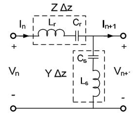
Fig 3. Distributed Impedance Model
