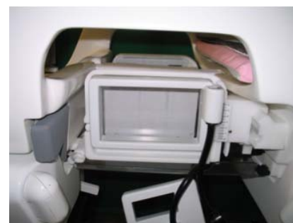
Figure 2: Vanguard Breast Biopsy table with a dual tuned coil.
