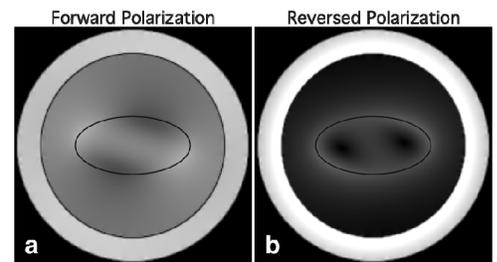
**Figure 1:** Simulated receiver sensitivity patterns at 1.5T for an infinite birdcage containing an elliptical load. Scattering fields induced by the load lead to signal inhomogeneity when the coil is phased for forward polarization (a), and regions of undesired sensitivity when polarization is reversed (b).
