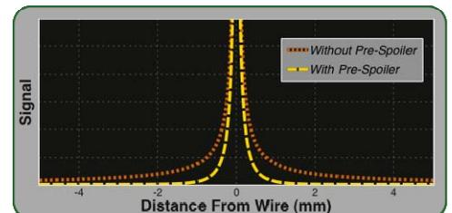
**Figure 3:** Wire signal as a function of distance from the wire shows that pre-spoiling has little effect near the wire, while signal further away is suppressed.
