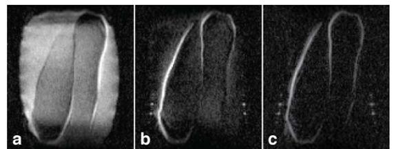
**Figure 4:** Projection EPI images of a wire lead in a 36-cm gel phantom. (a): Forward polarization; (b): Reversed polarization without pre-spoiler; (c): Reversed polarization with pre-spoiler. The added spoiler cancels residual background while retaining wire signal.
