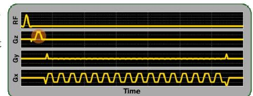
**Figure 2:** Pre-spoiled projection EPI sequence for detecting RF coupling. A reversed-polarization EPI readout detects RF wire currents. Signals arising from imperfect polarization reversal are suppressed by an extra z-spoiler (orange circle).
