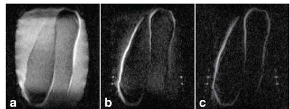
**Figure 4:** Projection EPI images of a wire lead in a 36-cm gel phantom. (a): Forward polarization; (b): Reversed polarization without pre-spoiler; (c): Reversed polarization with pre-spoiler. The added spoiler cancels residual background while retaining wire signal.
