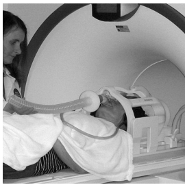
Mouthpiece, nose clip, and a rebreathing tube used to generate mild hypercapnia.
