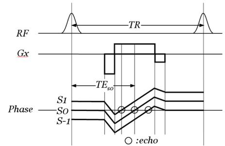
Figure 1. ME-SSFP with unbalanced gradients creates constant nonzero net phase dispersion in each TR cycle. In this study, three echoes are sampled corresponding to steady-states S<sub>1</sub>, S<sub>0</sub> and S<sub>-1</sub>.
