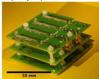
Fig 1: Photo of a stack of 3 PCBs with 12 parallel receive channels.
