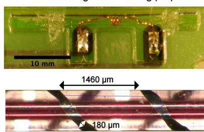
Fig. 3: Pictures of a wire coil in the holder and an inkjet printed silver coil.
