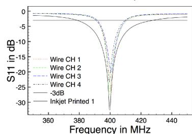
Fig. 2 Frequency response of four wire coils and one inkjet printed coil.
