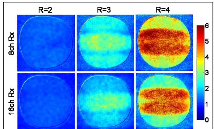
**Figure 2:** GRAPPA g-factor measurements for nominal reduction factors of 2, 3 and 4. For comparison, the conventional 8ch Rx coil results are shown in the upper row.
