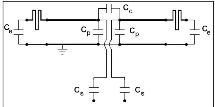
**Figure 1:** Electrical schematic of the improved strip line element with meanders. The capacitor  $C_c$  is the newly introduced decoupling capacitor to decouple the two branches of the element.
