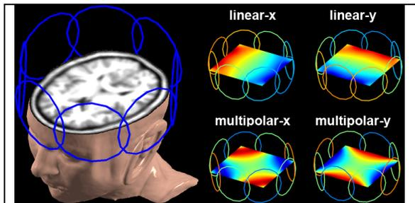
Figure 1. Left: The simulation setup of the 8-channel PatLoc system with an 8-channel RF coil array. Right: two pairs of spatial encoding magnetic fields (SEMs) used in PatLoc. This includes one pair of traditional orthogonal linear SEM and one pair of multipolar SEM.
