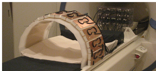
Figure 1: The 16-channel coil on the patient table. The two multipurpose T/R-switch and preamp boxes are visible at the bore opening.
