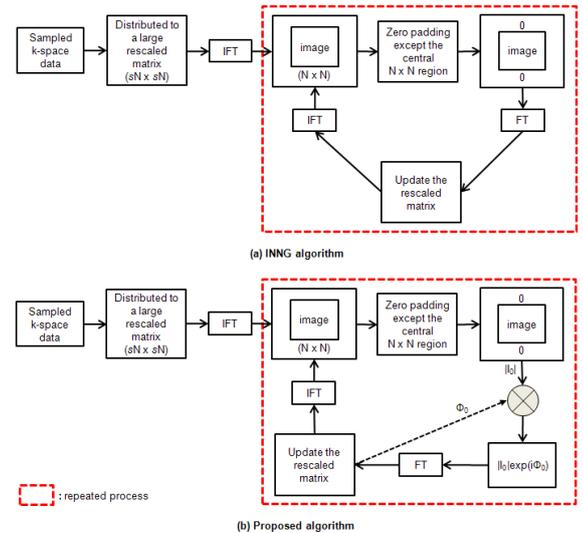
Figure 1: Flow charts of the (a) original INNG and (b) our proposed algorithm
