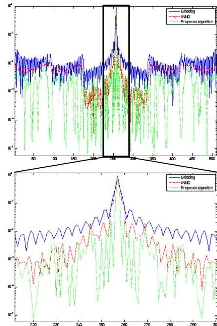
Figure 2: PSF profile (SD = 20%) of conventional gridding, INNG, and proposed algorithm. A logarithmic scale is used in the vertical axis.
