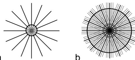
**Fig. 1** GROWL reconstruction scheme. (a) The original undersampled dataset with a small Nyquist circle. (b) After each radial view is widened into a band using a GRAPPA operator, the Nyquist circle is enlarged.
