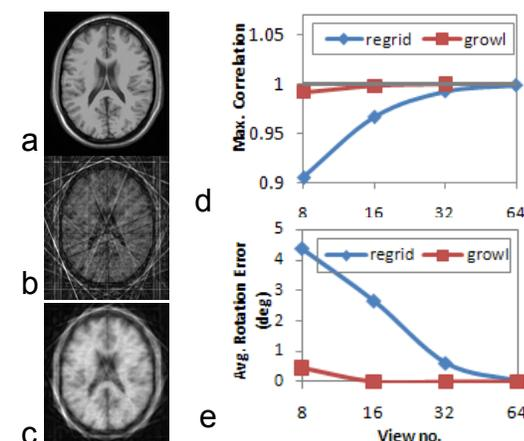
**Fig. 2** Simulation results demonstrating the motion detection accuracy of GROWL recon. (a)-(c): Reference image (a, 256x256), reconstruction using 8 radial lines with regridding (b) and GROWL (c). (d)-(e): Maximal correlation (d) and average rotational errors (e) with different no. of views.
