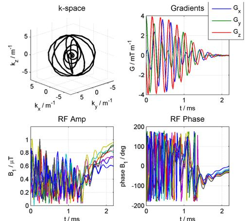
**Fig 1** K-space trajectory, gradients and optimised RF pulse (colours represent different RF channels)
