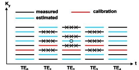
**Figure 1.** Undersampling pattern used for fast T<sub>2</sub> measurement (R = 2). The crosses represent the samples involved in the reconstruction of the missing sample (circle).
