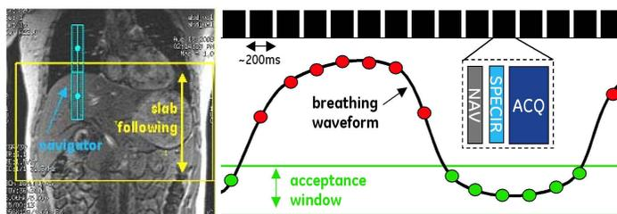
Fig. 1. (left) Navigator prescription and (right) navigator gated acquisition.
