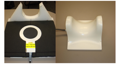
Figure 1: 7 T cervical spine coils. Left : single-channel loop. Right: 4-channel surface array.
