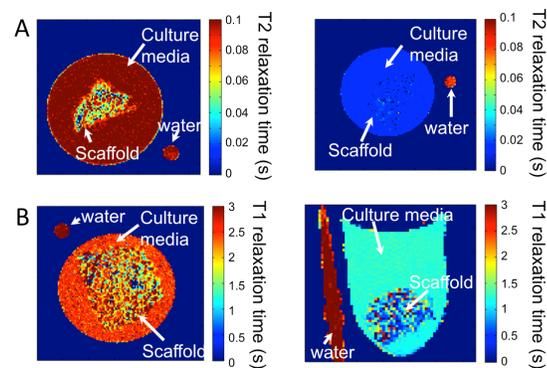
**Figure 2.** MRI of PPF scaffold and released nanoparticles (MRI was taken after 48h incubation).
