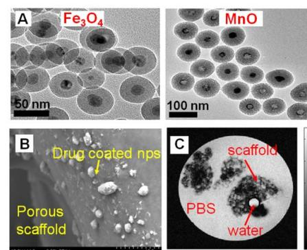
**Figure 1.** Nanoparticles' size and shape, PPF scaffold surface, MRI of PPF scaffold in PBS solution.
