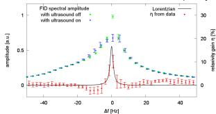
if ultrasound (US) matches Larmor frequency. These experiments were carried out using an NMR spectrometer where shielding of the receiving coils can be realized easily. In an MRI device, however, US radiation at MRI Larmor frequency would lead to disturbance of the MRI device.
