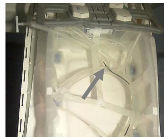
**Fig. 2:** Experimental setup with vessel model (silicone tubing) in water bath, receive body array coil, and inserted catheter (arrow).
