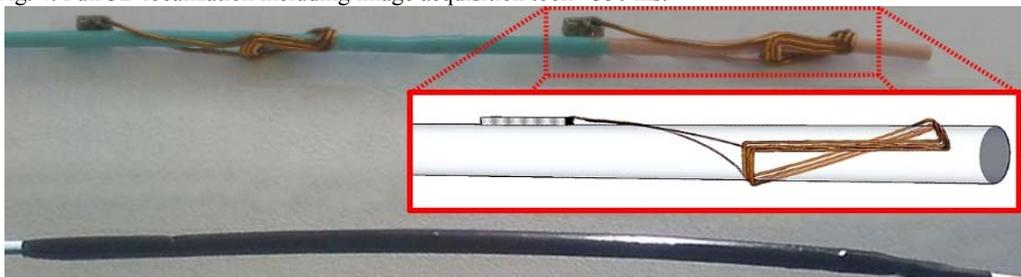
**Fig. 1:** Two inductively-coupled RF coils tuned to the resonance frequency of the MR scanner (63.8 MHz) mounted on a commercial 6F catheter. Schematic (inset) and actual (zoomed area) coil design with three non-planar turns of a 0.3-mm insulated copper wire and a ceramic chip capacitor. Bottom photo shows the tested design with the coils wrapped by a (medically grade) heat shrink tubing ( $\varnothing \approx 3.3$  mm).
