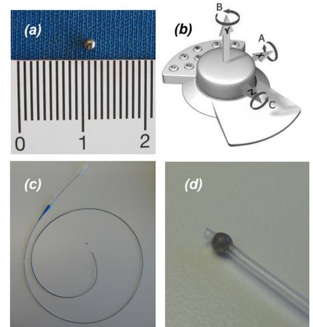
Fig 1. Ferromagnetic sphere (a) combined catheter (c) with a 3cm long 2mm thick silicon tube (d) and interactive control tool "space mouse" (b).
