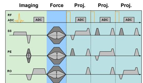
Fig 2. Schematic of the 2D FLASH navigation pulse sequence with force gradient and projections in all three spatial directions.
