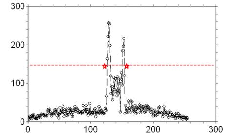
Fig 3. The center positions of the region (which was three times higher than the mean signal value) of the projection signal were calculated and supposed as positions of the tip.
