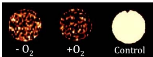
Fig. 1 T2 map of 50 mM ascorbic acid in anaerobic and aerobic solutions. At neutral pH (7.0) both O 2 -free and O 2 -enriched phantoms exhibit T2 shortening, although T2 and T2* effects are slightly increased in the presence of O 2 .
