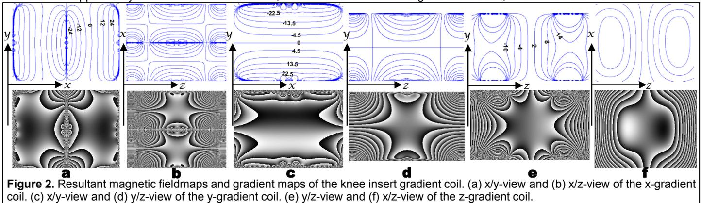
Figure 2. Resultant magnetic fieldmaps and gradient maps of the knee insert gradient coil. (a) x/y-view and (b) x/z-view of the x-gradient coil. (c) x/y-view and (d) y/z-view of the y-gradient coil. (e) y/z-view and (f) x/z-view of the z-gradient coil.
