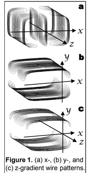
Figure 1. (a) x-, (b) y-, and (c) z-gradient wire patterns.
