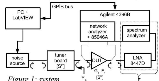
Figure 1: system diagram (curved arrows indicate reflections)
