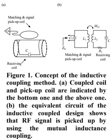
**Figure 1.** Concept of the inductive coupling method. (a) Coupled coil and pick-up coil are indicated by the bottom one and the above one. (b) the equivalent circuit of the inductive coupled design shows that RF signal is picked up by using the mutual inductance coupling.
