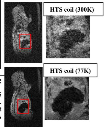
**Figure 3.** The images using 3D GEFI sequence to acquire. The slice thickness is 0.3125 mm. The SNR of HTSC is 23. And the SNR of HTS coil at 300K is 10. The SNR gain is 2.3 folds.
