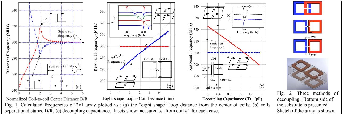
Fig. 1. Calculated frequencies of 2x1 array plotted vs.: (a) the "eight shape" loop distance from the center of coils; (b) coils separation distance D/R; (c) decoupling capacitance. Insets show measured  $S_{11}$  from coil #1 for each case.
