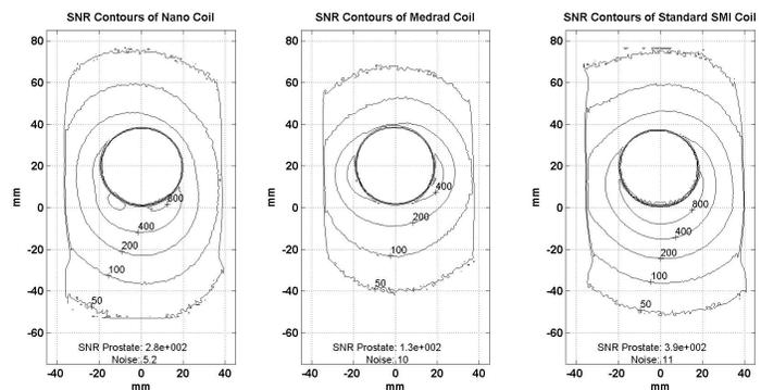
**Fig. 3:** SNR contours for the nanocoil (left), the Medrad coil (middle) and the standard Sentinelle dual-channel coil (right)
