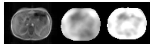
Fig. 4: RF Shimming for an 8-channel TX system: the image shows the target anatomy for the B1 maps (left), quadrature shim settings (middle) and adapted shim settings derived from the measured B1 (right).
