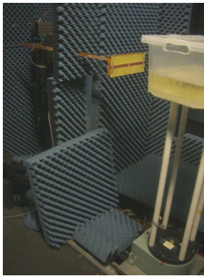
Fig.1 The measurement set-up for the “radiation plus sample-loaded” Q-factor is to be seen in Fig.1 where the coil is placed in our
