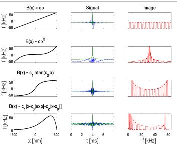
**Figure 2:** Simulation of position encoding with various curved magnetic fields results in region-dependent resolution properties of the encoding. Spatial encoding functions from top to bottom row: Linear; Cubic; arc-tangent; Rayleigh.
