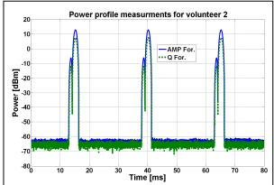
**Figure 2.** An example of the power profile for Vol2. A field echo sequence is used with TR = 25 ms.
