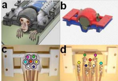
**Figure 1:** (a) Cartoon of the non-invasive restraint system. (b) Design of individualized helmet restraints. The helmets are composed of a head piece and a chin piece, which are lined up with foam to provide comfortable head support and restraint. (c) A 7-coil arrangement grooved on the inner surface of the head piece. All coils are symmetrically arranged in the head piece. (d) Top view of the helmet showing the coil circuitries and the  $\lambda/2$  RF cables.
