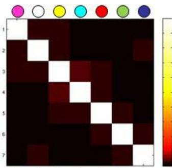
**Figure 2:** Noise correlation matrix. The highest off-diagonal correlation coefficient is 0.037.
