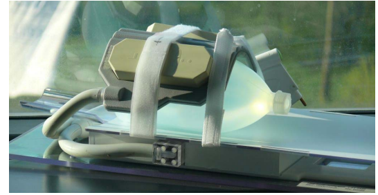
Fig. 1: Photograph showing the coil setup with a phantom bottle in the middle.
