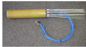
Fig.3. The constructed prototype of the 8-element transceive array coil
