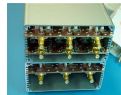
Fig.4. The 8-channel Tx/Rx switching/preamplifier unit
