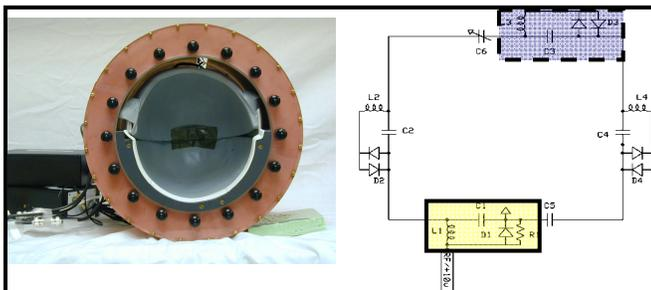
Fig. 1: (Left) Picture of the 16-element TEM Tx with 14-channel Rx-only insert and (Right) 1 element in Rx only array with passive & active decoupling (from the Tx coil) circuits.
