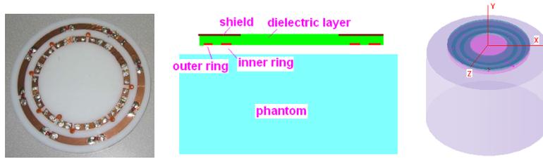
Figure 1. Two-ring coil prototype (left) and FDTD coil model placed 1cm-above a phantom (right).
