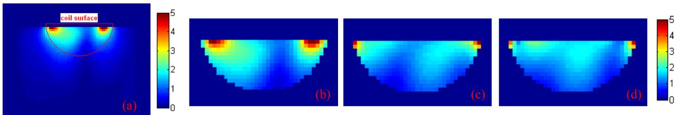
Figure 2. (a) Normalized  $|B_1^+|/|B_1^+|_{\text{center}}$  in the central transverse slice of the phantom from the inner ring only;  $|B_1^+|$  in a 17cm-diameter coil coverage area from inner ring only (b); from outer ring only (c); and from two-channel optimal driven (d).
