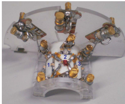
Fig. 2: 3-Channel receive array. The balun in the input circuit is mounted on the vertical plate.
